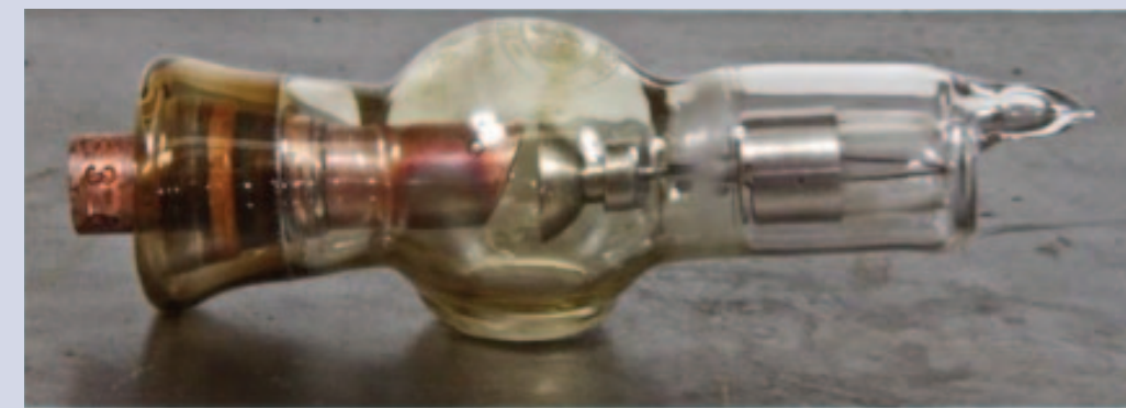
American Industrial Diminutive Medical "Victor" Portable Dental X-ray machine cylindrical glass Coolidge Tube. Circa 1920s.
